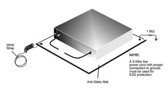
Figure 16. Typical configuration for ESD protection
